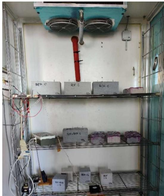
Figure 1 Environmental  $CO_2$  chamber hosting concrete specimens
